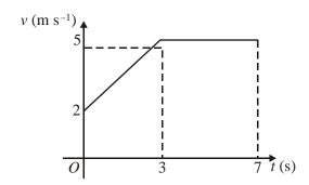
The figure above shows the speed-time graph of a cyclist moving on a straight road over a 7 s period. The sections of the graph from t = 0 to t = 3, and from t = 3 to t = 7, are straight lines. The section from t = 3 to t = 7 is parallel to the t-axis.
