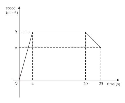
A sprinter runs a race of 200 m. Her total time for running the race is 25 s. The diagram above is a sketch of the speed-time graph for the motion of the sprinter. She starts from rest and accelerates uniformly to a speed of 9 m s<sup>-1</sup> in 4 s. The speed of 9 m s<sup>-1</sup> is maintained for 16 s and she then decelerates uniformly to a speed of u m s<sup>-1</sup> at the end of the race. Calculate
